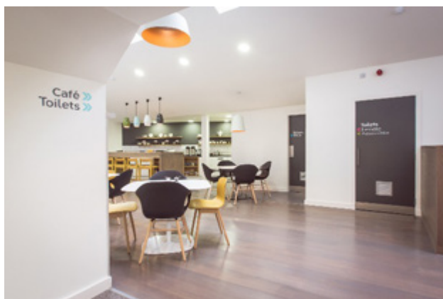
The entrance to café demonstrates the solid colour flooring, excellent light levels and non-confusing wayfinding. Text rather than images is used on toilet doors, as the demographic is proportionality living well with their illness and decided not to use images as this presents a more significant vision of future need.
