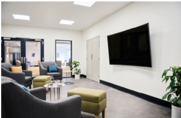
The TV room is separated from the lounge room to avoid loud noises. Black skirting was selected to give contrast between wall and floor. Residents use doors that have black frames while white frames signify no use.
